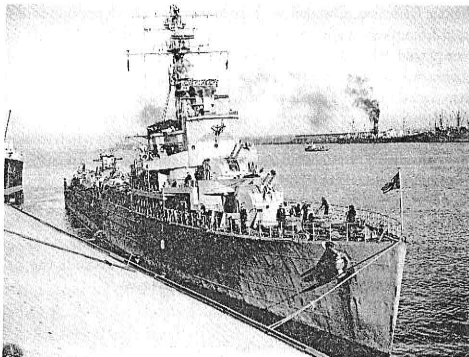
Figure 3: The anti-aircraft cruiser Jacob van Heemskerck at Fremantle, date unknown. Still incomplete when the Netherlands was occupied by Germany in May 1940, the Tromp-class ship was towed to Britain, where it was completed to a modified design with a main armament of British 4-inch anti-aircraft guns. [Courtesy of the family of Saxon Fogarty and Fremantle Ports]
